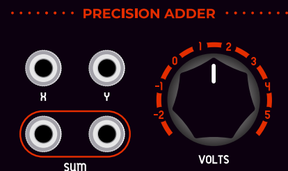
Fig.3 Detail of Precision Adder Utility Module
